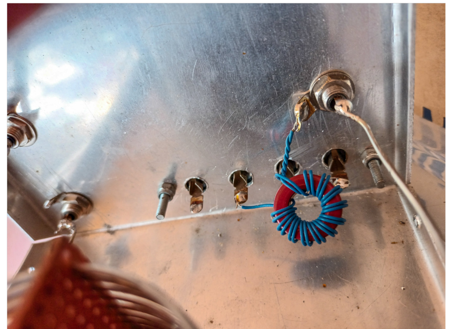
Inside view of front connections and Balun placement
